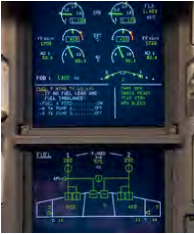
(fig.2) Low level alert display on ECAM
